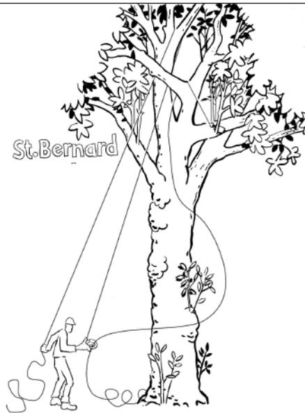
**1.-2. Using a second throwline (the first one is stuck in the tree), throw into a crotch somewhere above the stuck throw weight. Remove tw2 from the second throwline, tie on a carabiner, and clip the carabiner around the first throwline.**
