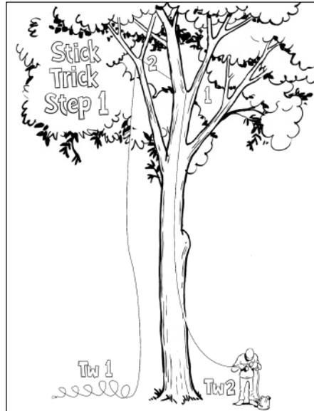
1. Tie the end of the rope to a dog-leash snap. Use a knot that is fairly large and heavy, such as a bullet knot, monkey's fist, throwing knot, or tightened hangman's noose.
