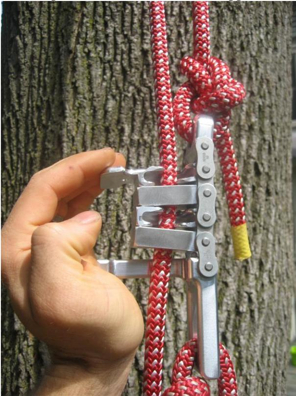
Squeeze against the lower handle with your palm while holding the rope exiting the bottom of the UNICENDER climbing tool with the other hand down by your hip.
