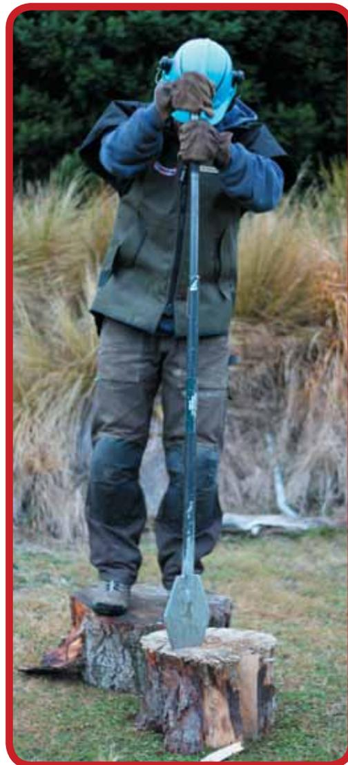
Split from the outside using the blade with the grain for large rounds and in half for small rounds.
