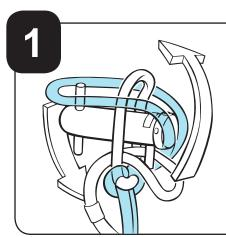
SLING ATTACHMENT Attach mooring sling to long loop (sling loop) of Portawrap by threading the sling's eye through then passing over the device to create a secure cinching hitch.
