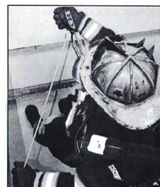
Once device is loaded, both hands are needed for operation: brake hand must be on free end of rope. Descent is controlled by squeezing release lever and varying pressure on free end of rope with brake hand. To stop, let go of release lever.
