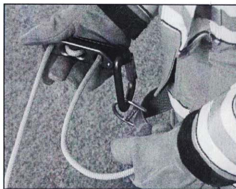
For horizontal movement, squeeze release lever, and while moving horizontally, hold the F4 parallel to the floor and at a 90 degree angle to the anchor. Rope will be fed into the device from storage allowing the device will slide along the rope.
