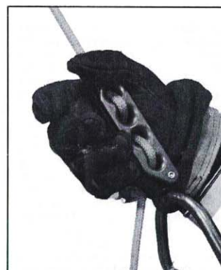
Squeeze lever to begin descent, with brake hand on the free end of rope.
