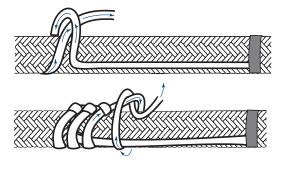
Continue with this procedure until the whipped area is approximately 1/2 of the desired length, then cut off the taped end near the last wrap.
