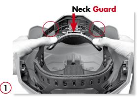
Push the neck guard towards the inside of the helmet until it snaps into place (with a slight click). In this position you can see the right and left adjustment straps (see circle Fig. 3). Use these to adjust the Protos® Integral safety helmet to your head size.
