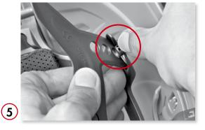
Push the adaptor button towards the outer shell. Now you can select one of the three ride heights by pushing the button in our out. Here, too, make sure to make the same adjustments on both sides!
