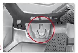
Take the ear protection incl. bracket and slide it into the corresponding clasp.
