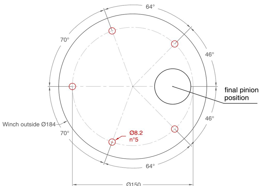
**B.** Remove the winch and drill the five 8.2 mm diameter holes.
