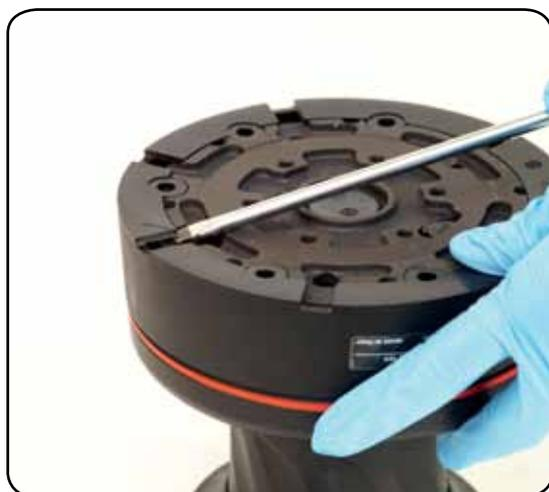
1. Remove the skirt n°2 with the help of the screwdriver placed as shown by the symbol
