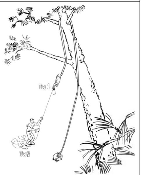
7. Pull tw2 into the tree so that it catches the dog-leash snap, and pull the rope to the ground.
