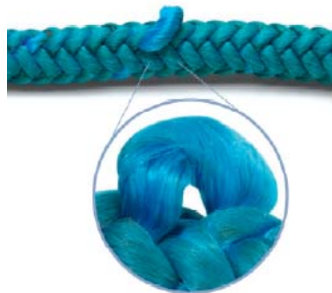
Rope with a Pulled Strand
