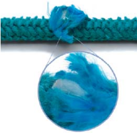
Rope with Broken or Cut Strands
