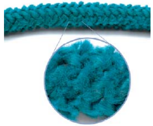
Rope with Excessive Abrasion Wear
