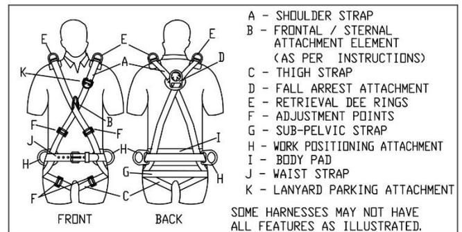
NOTE: Lanyard parking attachment is not to be used as a load bearing anchor point.
