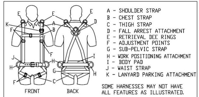
(FIGURE "A") Pick up your harness by the fall arrest attachment (item 'D') and shake it to allow the straps to fall free of each other. Make sure the leg strap buckles are unbuckled at this time. At this point, you will note the different colors of the webbing. The leg straps and the shoulder straps will be a contrasting color. Kevlar harnesses will have a contrasting colored stripe on the leg and sub-pelvic straps to distinguish them from the shoulder straps.
