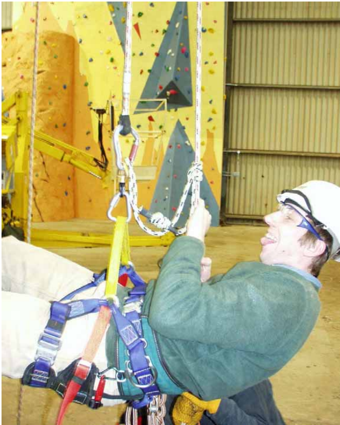
Figure 5 – Poor attachment of prussik loop.
