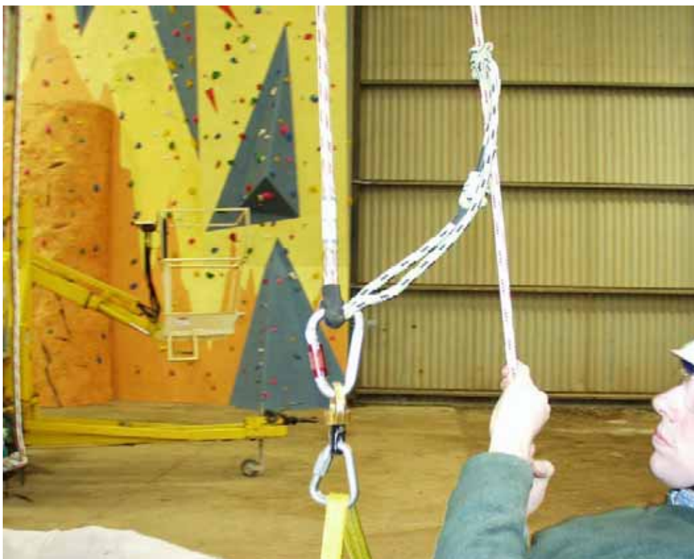
Figure 8 – Prussik loop held by plastic clip.
