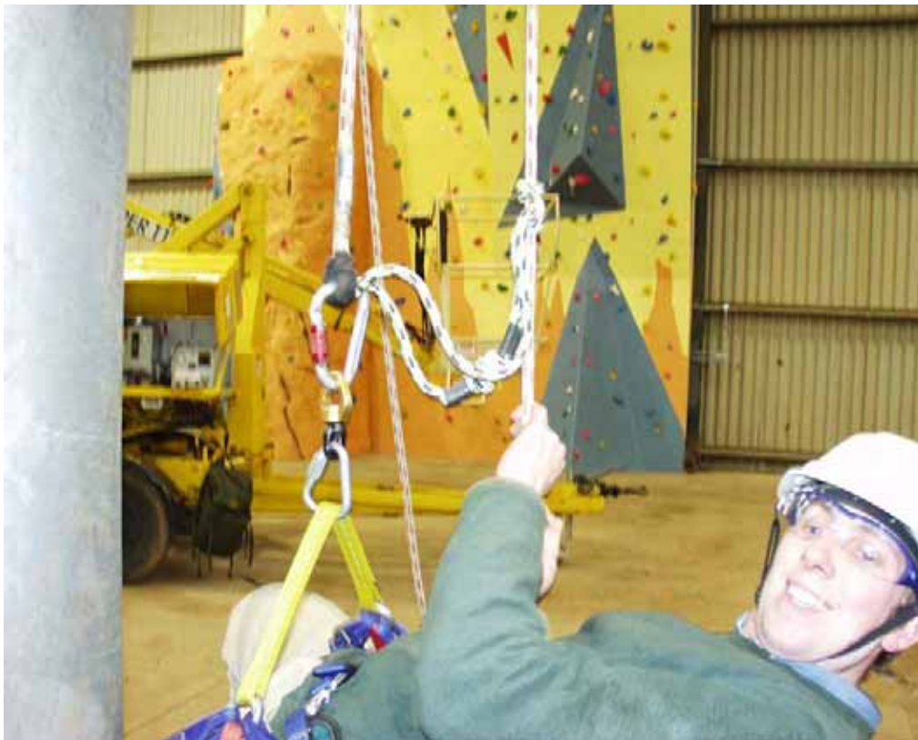
Figure 7 – Prussik loop held by elastic band.
