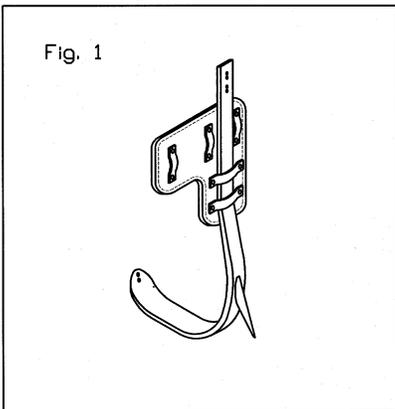
Attach sleeve to leg iron with sleeve loop facing outside of pad (away from the wearer's leg) using the fasteners enclosed. See Fig. 2 ('right' climber shown). **Note:** Two fasteners (screws, star washers & barrel nuts) must be used to secure each sleeve to each leg iron. Do not over tighten, torque to 25 inch pounds maximum.
