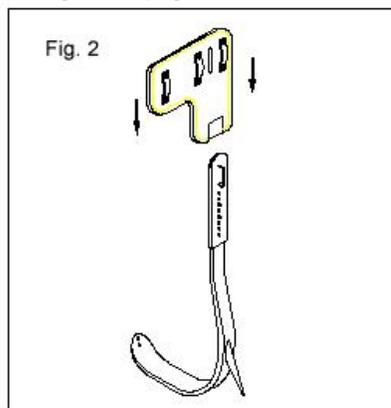
Slide the climber pad along the shank of the climber onto the sleeve, aligning the sleeve loop with the loops on the horizontal leg of the pad. Insert climber strap in the direction shown, through the pad loops and the climber sleeve loop. See Fig. 3 ('right' climber shown). **Note:** Foot strap must be attached to the leg iron stirrup in the same direction as shown for the calf strap.
