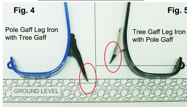
Gaff lengths when measured on the underside should not be less than 1-1/4" for pole gaffs or 2 1/4" for tree gaffs. When not being used for climbing, climber gaffs must be protected with gaff guards.
