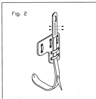
Slide the climber pad along the climber sleeve onto the climber, aligning the sleeve loop with the loops on the horizontal leg of the pad. Insert climber strap in the direction shown, through the pad loops and the climber sleeve loop. See Fig. 3 ('right' climber shown). **Note:** Foot strap must be attached to the leg iron stirrup in the same direction as shown for the calf strap.
