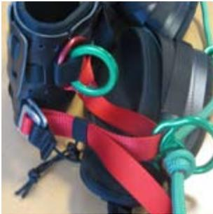
10. Pass the webbing through the loop of elastic material again. Before proceeding, ensure that all parts are in the correct place, are not twisted and that the buckles function correctly.
