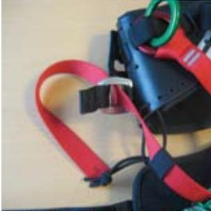
7. Ensure that the two adjustable buckle parts are sitting correctly. Pass the webbing through the slot closest to the waist belt.
