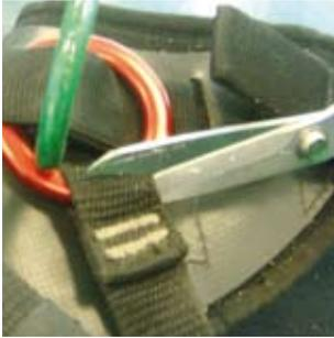
1. Remove the used connection being careful not to damage any other part of the harness.
