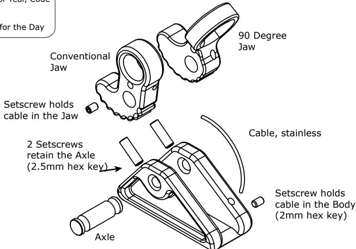
Always be sure cable is in good condition & provides a proper spring action & that the jaw operates freely over its whole range of travel.
