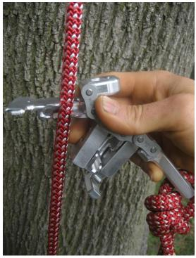
• Now hold the next clamping block away from the first and third to expose its slot. This slot is on the other side of the block. Bend the rope to allow it to slide into that slot.
