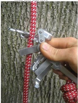
• Proceed in this manner inserting the rope into the alternating slots all the way to the last one.
