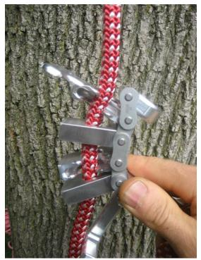
• Then position the rope within the "L" of the bottom handle.
