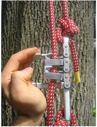
Squeeze against the lower handle with your palm while holding the rope exiting the bottom of the UNICENDER climbing tool with the other hand down by your hip.
