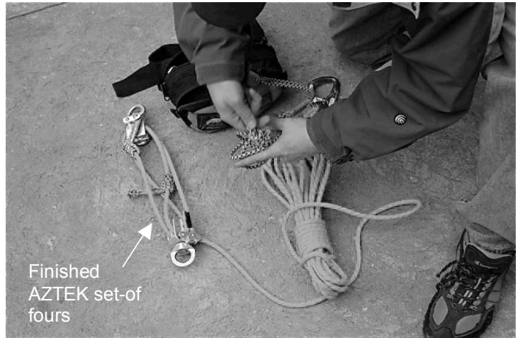
14. Pin in place orange ratchet to orange pulley or blue ratchet to blue pulley. DO NOT attached orange ratchet to blue pulley or vice versa. Only one ratchet should be attached at a time for proper operation.
