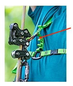
When you disconnect the chest harness to continue your work after an ascent, never leave the carabiner attached to the Rope Runner Pro SRS attachment point.
